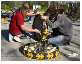
Experience: The steel construction worked well, however, the pre-tensioned leaf springs jumped out of their bracket from time to time and the tire was not rough enough and therefore offered little road grip. Added to this was the heavy weight, so the wheels proved to be somewhat impractical.
